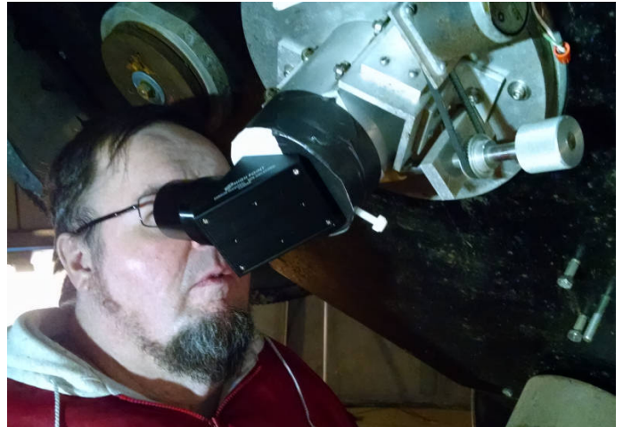
The author testing the eyepiece position in the mock-up. There is enough room for comfortable viewing even when using the "wrong" eye, and with the 40" mirror, the central star of the Ring Nebula is imagined to be easily visible in the view.
