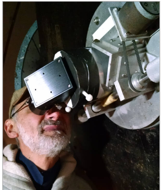
The author testing the eyepiece position in the mock-up. There is enough room for comfortable viewing even when using the "wrong" eye, and with the 40" mirror, the central star of the Ring Nebula is imagined to be easily visible in the view.
