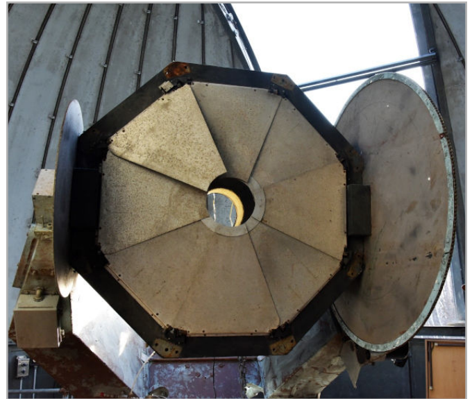
Front view of the instrument with the truss removed, featuring the mirror cover.
