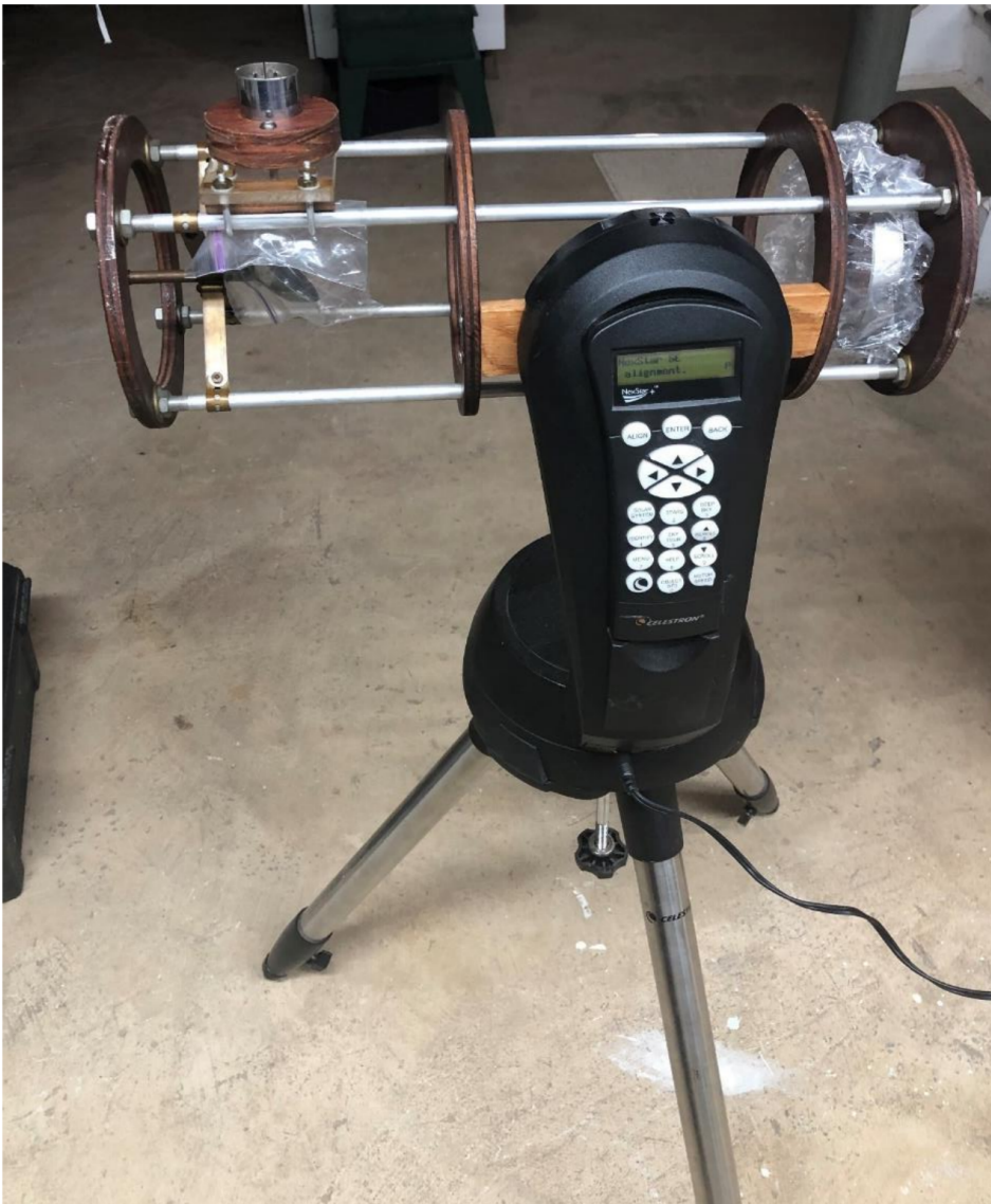
3. ShenkleScope mounted to Celestron single fork-arm go-to mount.
