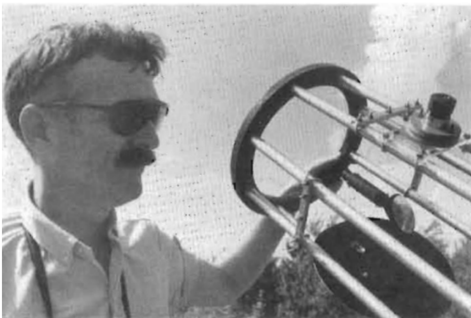
Left: Paul G. Shenkle's 8-inch f/5 Newtonian won second prize for optical excellence. The diagonal is supported in the open-frame tube by 8/1,000 piano wire. This reduces diffraction and improves planetary contrast. The tube is made of aluminum tubing supported by Masonite rings. Mr. Shenkle is a member of the Lehigh Valley Astronomical Society, Allentown, Pennsylvania.
